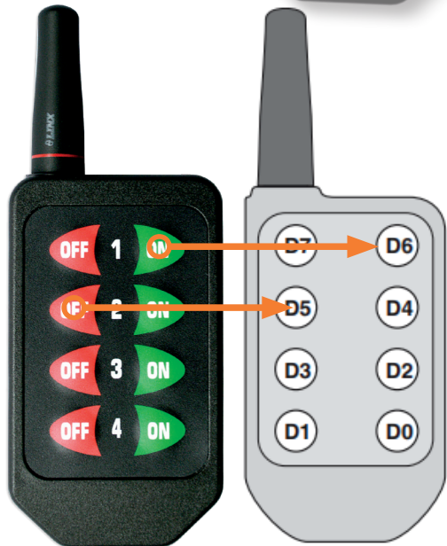
Key Fob buttons as they are related to the internal DIP Switches.
